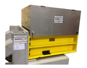
Brelx provides factory performance test for all sizes of Rail Clamps. So called "Push Test" is completed in our factory on the actual rail clamp.
