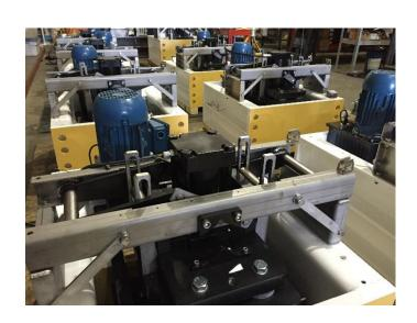
BRELX Rail Clamp on a test stand
